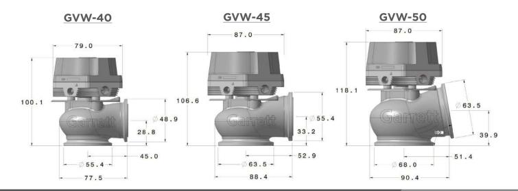
External wastegates for turbocharged racing and performance engines
